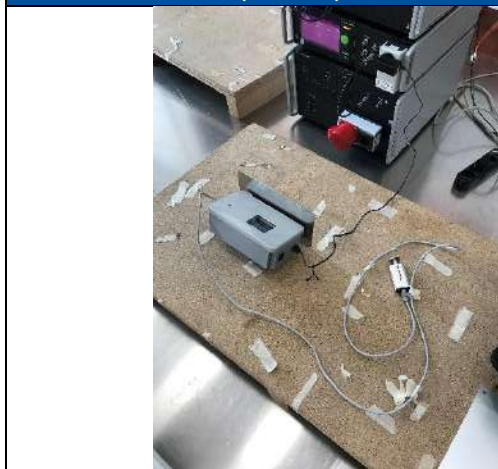
PHOTO 5 – BURST/SURGE/DIPS IMMUNITY SETUP
